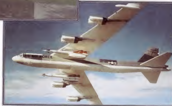
▼ Hound Dog carrier As ICBMs (intercontinental ballistic missiles) became more important, the B-52 took on the launching of stand-off weapons such as the jet-powered AGM-28 Hound Dog missile.
